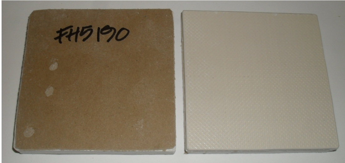
Figure 1 Representative specimens (unexposed face on left, typical exposed face on right)
