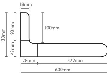
Having determined the dimensions of each component, prepare the blanks and laminate, then bond together ensuring that a spacer block is used to guarantee an exact dimension between the benchtop blank and splashback component.
